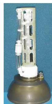
Measuring salinity on an Argo Float
