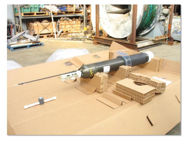
A regular argo float is a steel cylinder about 2m high. It contains a battery, a buoyancy device, measuring equipment and a satellite antenna. Image: M. Walkington, NIWA.
