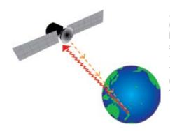
A further refinement to the answer is obtained by deriving a correction to the receiver's clock. This is done by deriving simultaneous measurements to at least four satellites. This means the receiver must have at least four channels. To get all the ranges (distances) from the satellites to meet at the one point the receiver will derive a correction which is applied as a correction to the receiver's clock.
