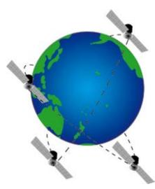
GNSS (Global Navigation Satellite Systems) essentially make use of numerous (a constellation) navigational satellites circling the earth to derive positions or navigate on the earth's surface.
